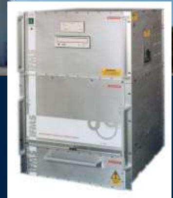
ESA's current deep space TTC modem
